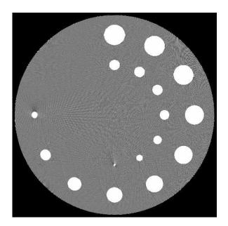
FIGURE 10. Reconstruction of the clock phantom from trajectory (5.2): slice z = 0, WL=0 HU, WW=100 HU.
