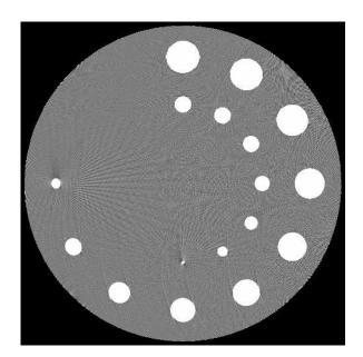
FIGURE 8. Reconstruction of the clock phantom from trajectory (5.1): slice  $x_3 = 0$ , WL=0 HU, WW=100 HU.
